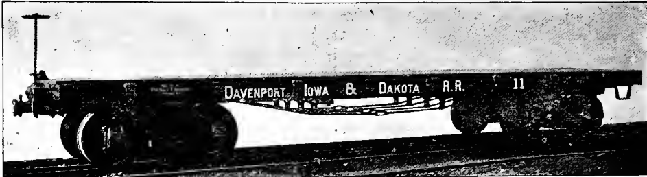
Fig. 18. FLAT CAR. DAVENPORT, IOWA & DAKOTA RAILROAD. Length, 34 ft. Capacity, 40,000 lbs. Weight, 17,700 lbs. Equipped with Rigid Diamond Trucks.
